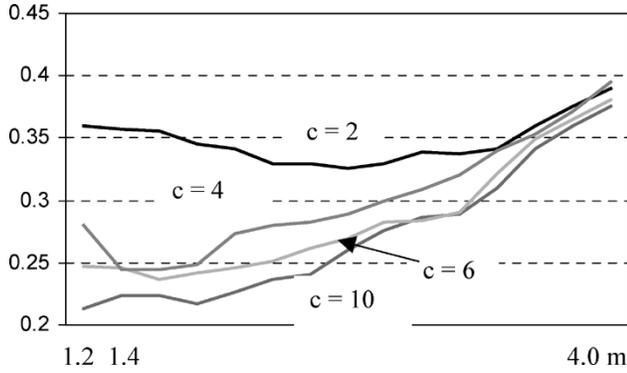
Fig. 7. Performance (granulation) index of the mapping as a function of the fuzzification coefficient of the FCM for selected number of the clusters ( $c$ ).
