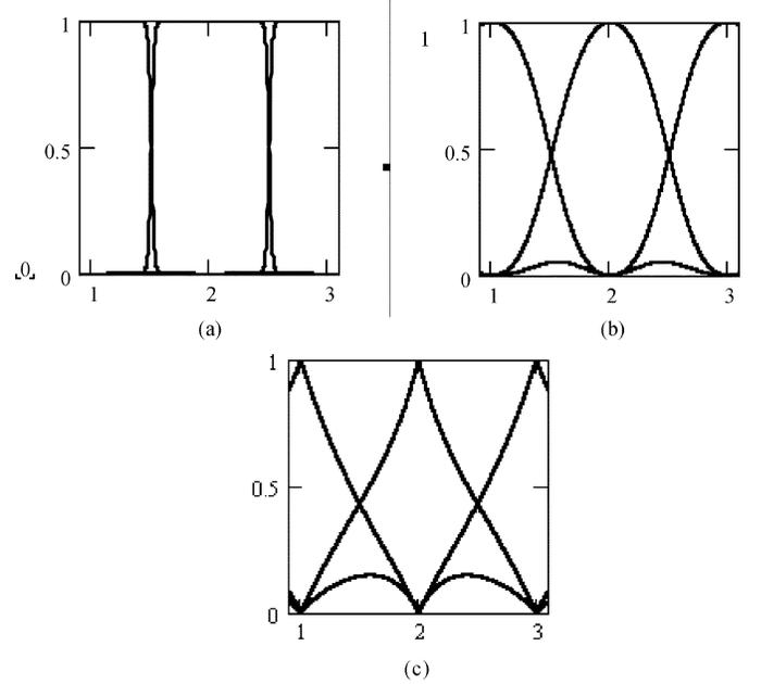
Fig. 6. Plots of membership functions of information granules generated by the FCM clustering for selected values of  $m$ : (a)  $m = 1.1$ , (b)  $m = 2.0$ , and (c)  $m = 3.0$ .
