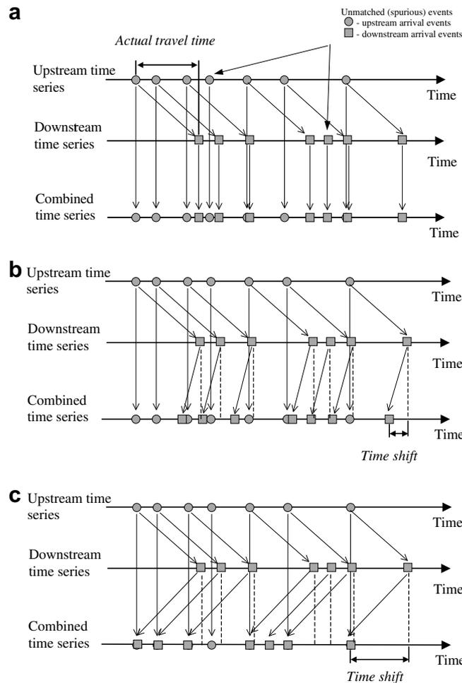
Fig. 2. Heuristic for estimating travel time by varying “Time shift” and evaluating the resulting matching of the two time series.
