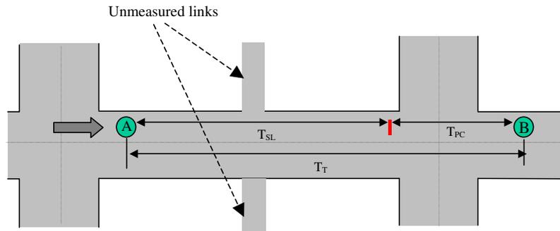
Fig. 1. Urban link model with upstream measurement (A), downstream measurement (B) and two unmeasured links.
