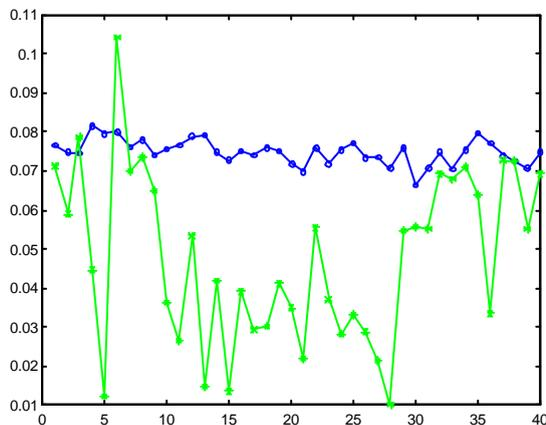
**Figure 6.** Reduction of the ratio of the volume of exclusion to inclusion hyperboxes (the ratio calculated originally for  $\Theta=1$  is plotted as blue “o” marks and the ratio obtained after adaptive shrinking of exclusion hyperboxes is plotted as green “\*” marks)
