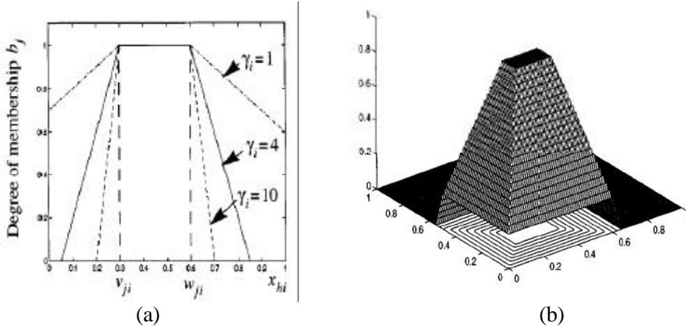
**Figure 1.** One-dimensional (a) and two-dimensional (b) fuzzy membership function evaluated for a point input pattern  $X_h$ .
