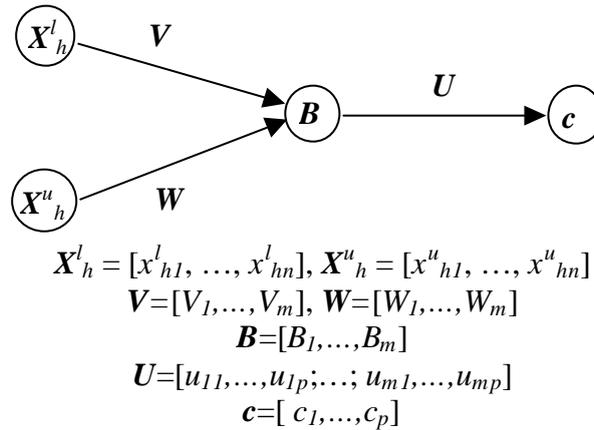
**Figure 2.** The three-layer neural network implementation of the GFMM algorithm.
