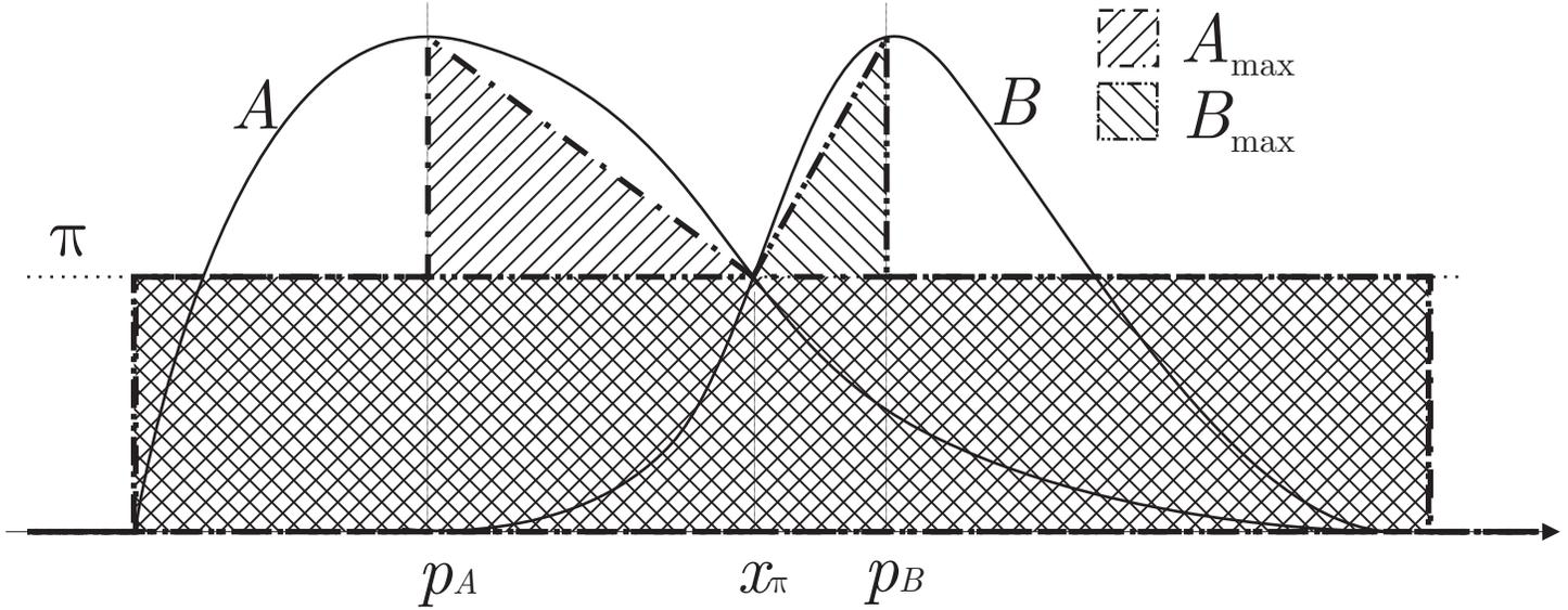
Figure 1: Example of fuzzy sets with maximal similarity for a given possibility measure
